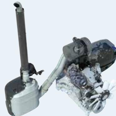
DIESEL ENGINE AFTER TREATMENT SYSTEM
